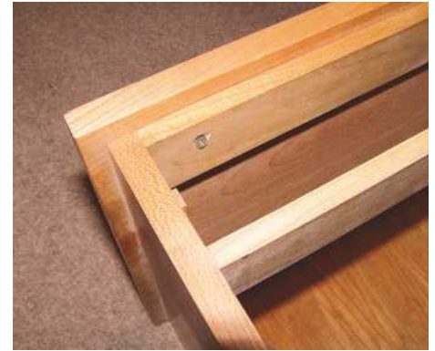
▲ Pic.15 The top panel was attached with screws, countersunk so as to clear the drawer back panel
